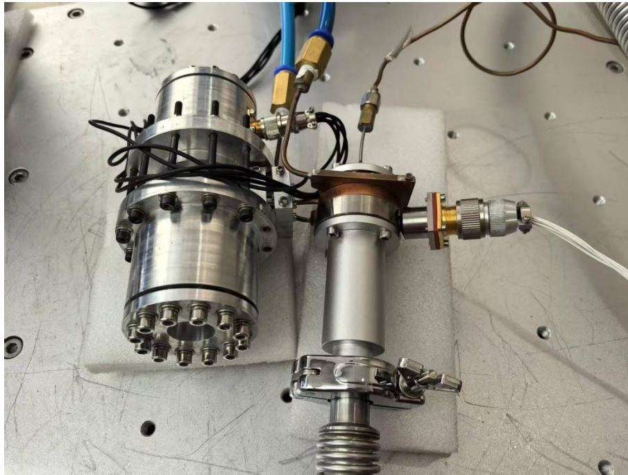
Figure 4. The pulse tube cryocooler prototype.
